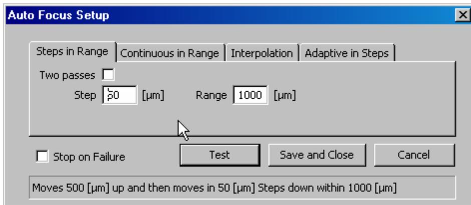
There are four Auto focus routines available in NIS-Elements, depending on the Z motor hardware installed on the system. Some routines are not available with certain Z devices.
